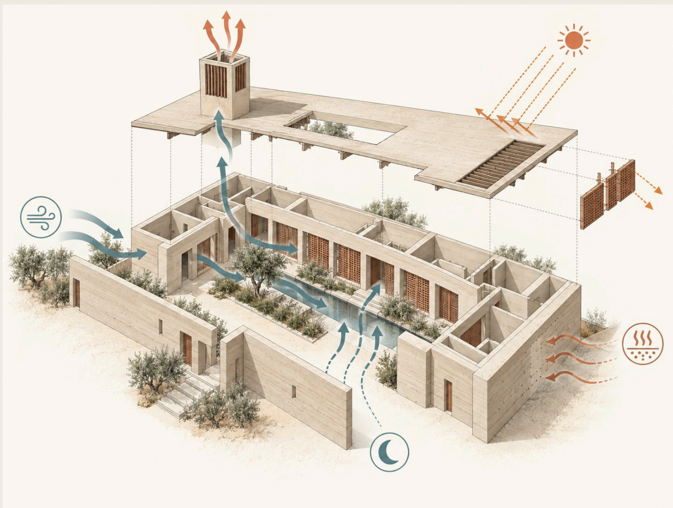
FIG. 03 · The environmental sequence: shade, air path, stack exhaust, thermal mass and night purge. Explanatory concept diagram; performance not yet simulated.
