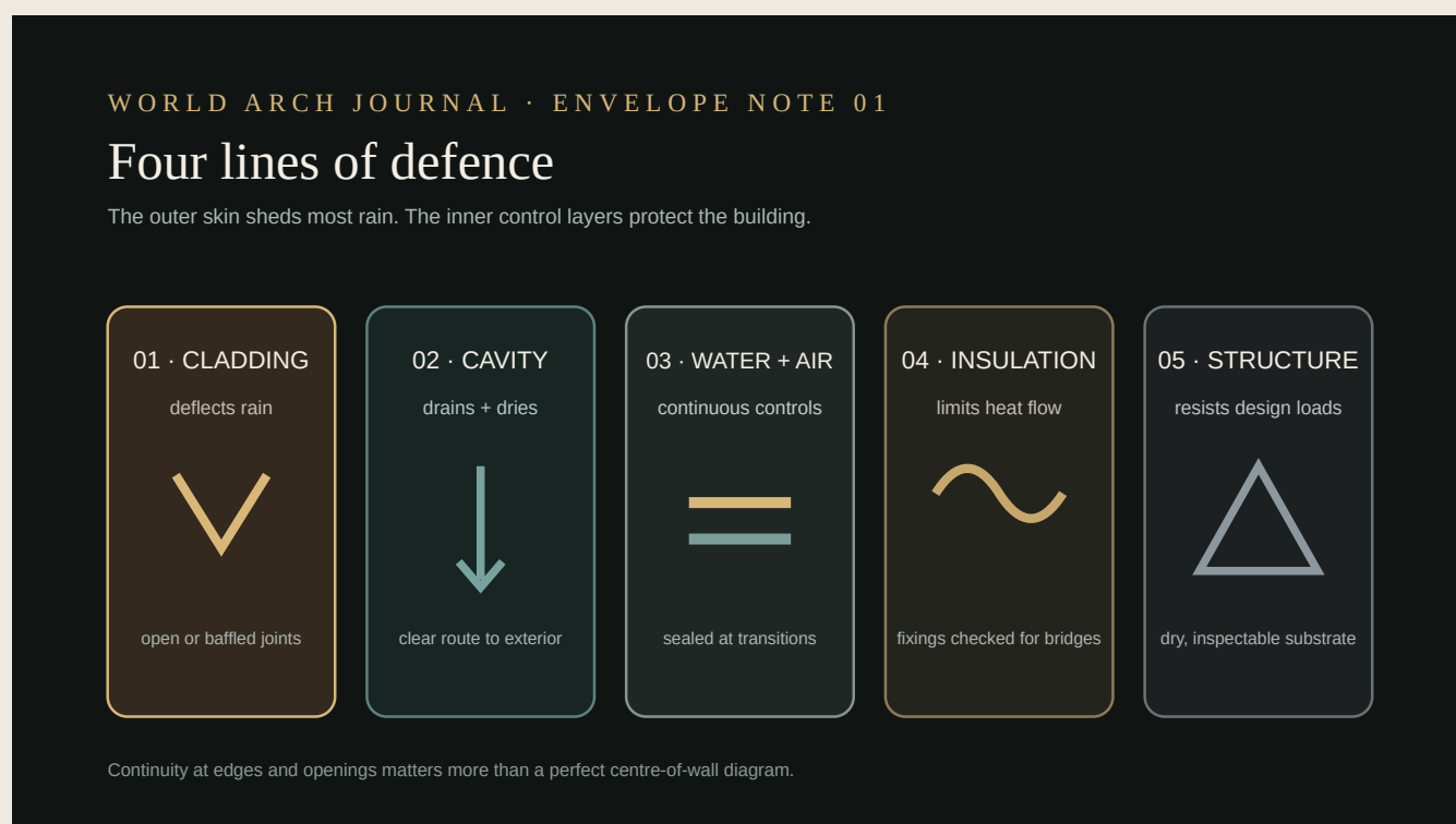
FIG. 02 · FOUR CONTROL LINES OF A RAINSCREEN · ORIGINAL WORLD ARCH JOURNAL DIAGRAM.
